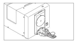
2. Remove the currently attached target mask by pulling it toward you.
