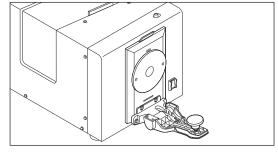
2. Secure the specimen with the sample holder.
