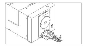
2. Fit the projections of the zero calibration box into the grooves on the CM-3700A and then close the sample holder to hold the box in place.
